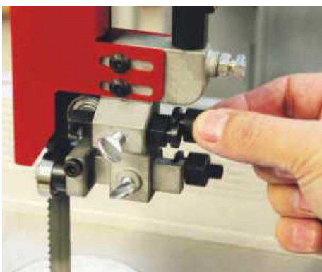
The upper guides are adjusted without the need for tools
